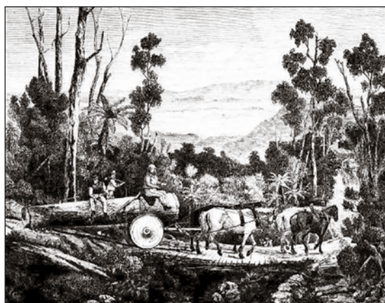
'Hauling Timber, Mount Macedon': sketch in Illustrated Australian News of February 1851. View from near the top, looking towards Dandenong Ranges. Having one end of the log dragging on the ground served as a brake on the steep timber trails.
