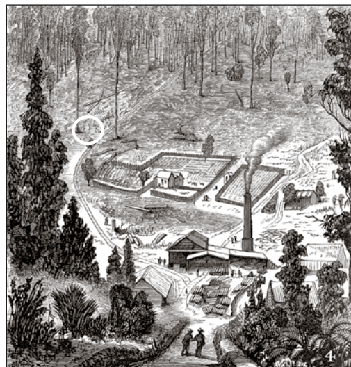
This illustration is of the Devil's Hole sawmill as it was in operation in 1874. Note the sawn log at left (circled) descending the slope on a tramway.
